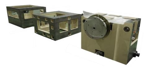
**BOX1** Upper wheel head. ~ Main body in cast iron BOX 2 Hood / wheels cover. Cast iron structure Lower wheel head BOX 3 Machine bed in cast iron
